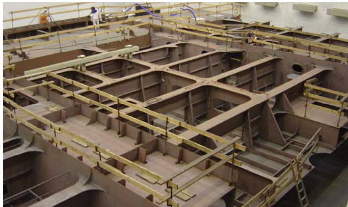
A ship section at the combi hall for the 'one-stop shop' process. Dimensions: L x W x H = 38 x 38 x 20 meter.
