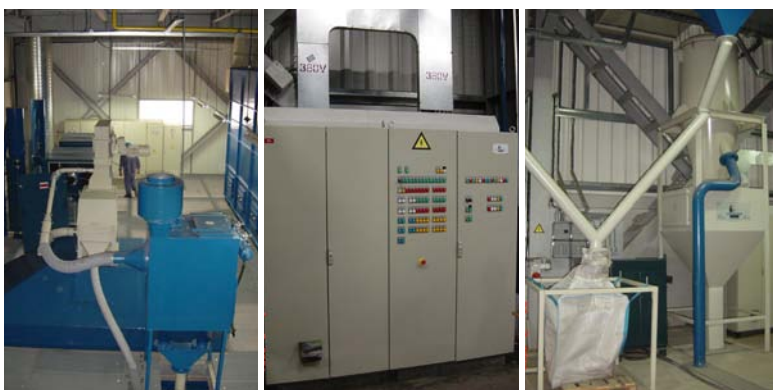
Left to right: Silo cleaning unit, PLC control box, Pre-separator
